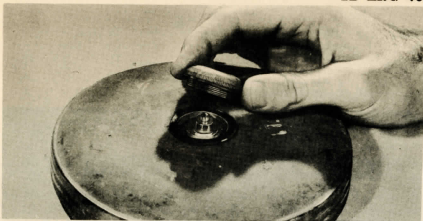
① Unscrewing brass pressure plug.
