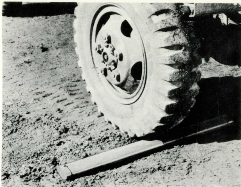
Figure 16. Yardstick mine used against vehicles.
