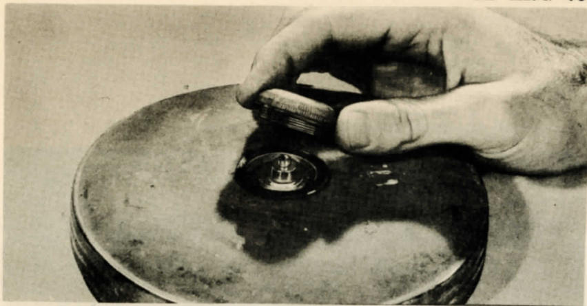
① Unscrewing brass pressure plug.
