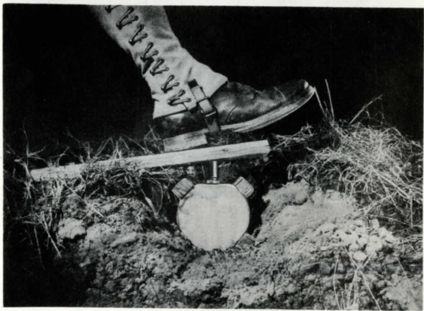
Figure 11. Using plank or board with magnetic mine to give more bearing on fuze.
